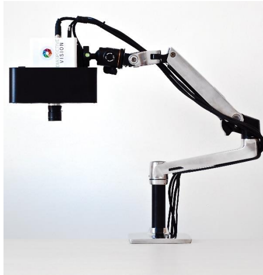
Figure 5: TIVITA® Tissue system with integrated lighting unit
